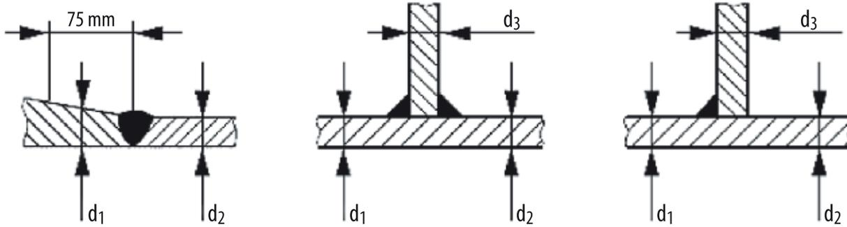
$d_1$  = Average thickness in 75mm long section. Combined plate thickness =  $d_1 + d_2$
